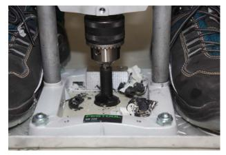
Insert repair patch D 35 (thickness 6,5 mm) with chamfer faceup.
