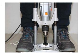
Insert cylinder head drill bit Ø 35 into drill. Check drilling depth (6mm) before drilling.
