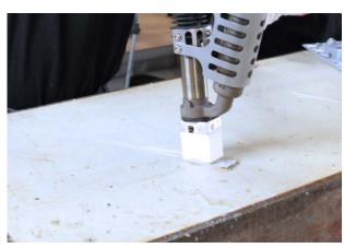
Protruding material is planed with a paint remover  $\dots$
