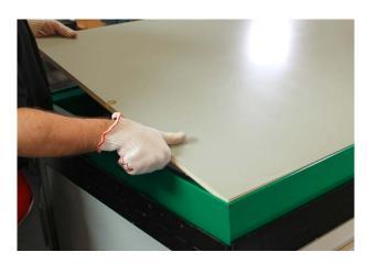
Guides are placed in the anchor holes in order to align the panel in the panel formwork.
