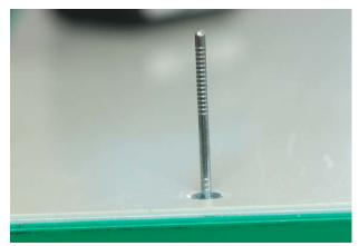
Use a pneumatic rivet gun to fix the rivets.
