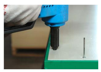
Since the alkus® panel neither swells nor shrinks, it is installed 'flush' into the panel formwork. This guarantees a perfect joint pattern from the very first use.
