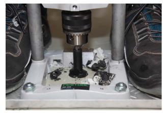
Insert repair patch  $\emptyset$  35 (thickness 6,5 mm) with chamfer faceup.
