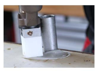
After the repair cone is removed, the repaired area is smoothened with a paint remover and paint scraper.
