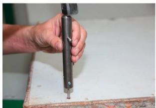
... then remove rivet by using a hammer.
