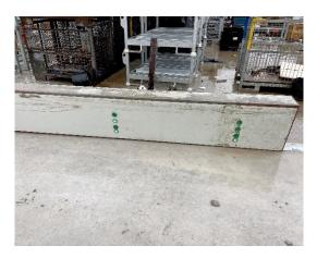
After 10 uses: The alkus® formwork panel with the alkus® sealing cones in the Peri formwork system. | © Bold GmbH & Co KG
